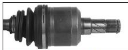
Inboard splines of non-locking differential CV
