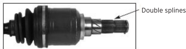
Inboard splines of locking differential CV
