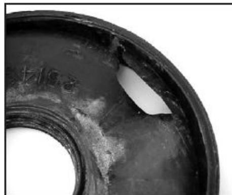
Typical vacuum booster diaphragm failure due to gas or gasoline fumes
